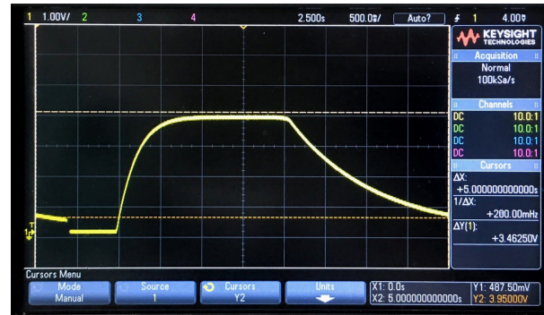
Figure 11: Successful microphone circuit response curve.
