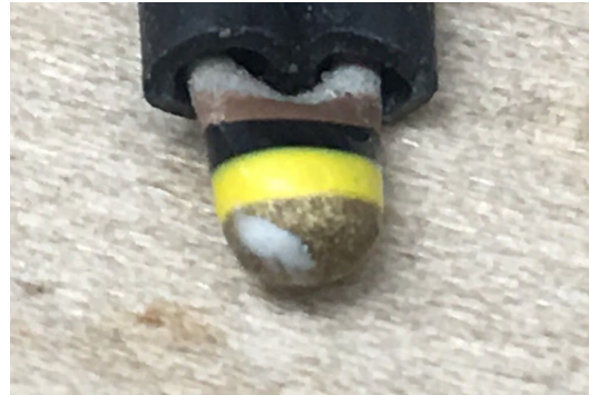
Figure 18: Thermistor with exposed metal wire near heat shrink.
